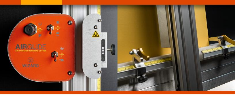
The Wizard AirGlide™ is a straight-line material cutter, powered by compressed air, that easily cuts the substrates you use most. The AirGlide features a 65" vertical cutting capacity with cutting and clamping mechanisms that are completely air-powered—no electricity is needed.
